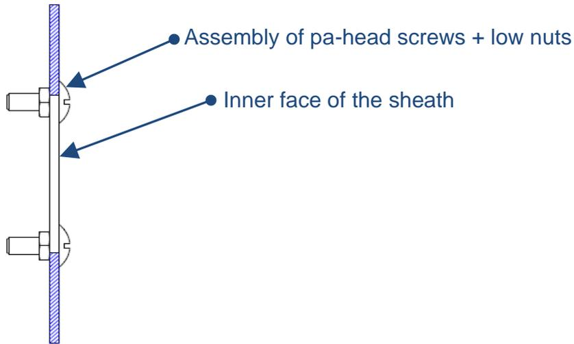
3) Adjust the trigger distance of the VIGIBELT® TOUCH detectors. This distance corresponds to the dimension between the inner wall of the elevator and the contact face of the detector.
